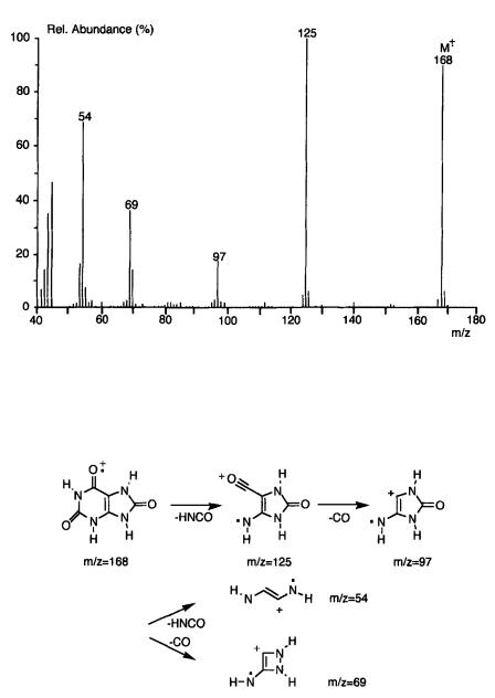
FIG. 3. Mass spectrum (EI, direct inlet, 70 eV, 220-400°C; Finnigan MAT 95) and characteristic fragmentation ions of the pheromone.
