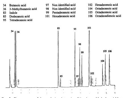
FIG. 5. Chromatogram of the synthetic mixture (condition 1, see Methods and Materials). Unidentified acids (numbers 97 and 98) were trapped by micropreparative gas chromatography from the total extract and added to the synthetic mixture.
