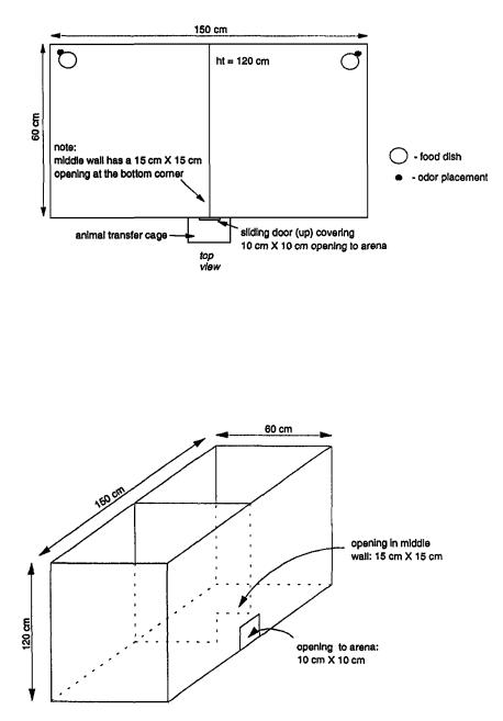
FIG. 1. Laboratory testing arena design for evaluation of predator odors to elicit an avoidance response in the roof rat (not to scale).
