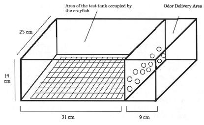
FIG. 1. Plexiglas test tank in which all experiments were performed. Intact items or bathwater leachates were placed into the odor delivery area, mixed, and allowed to diffuse through the porous partition and into the area of the test tank occupied by the crayfish.
