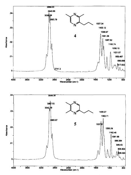
FIG. 2. GC-FTIR spectra of the dimethylpropylpyrazines 4, 5, and 6.
