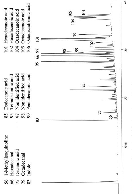
Fig. 3. Chromatogram of fraction 3 obtained from the total extract of dog feces (conditions described in Collection of Capillary Gas Chromatographic Fractions in Methods and Materials).
