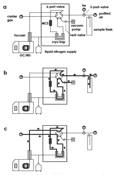
FIG. 1. Schematic diagram of the PCT/GC-MS arrangement (a) and gas flows during sample desorb (b) and trap desorb (c) steps.
