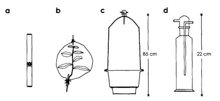
FIG. 2. Possible vessels for sample storage during headspace sampling: (a) glass tube, 6 mm OD, for single small specimens; (b) PET-film tube with 6-mm glass tube adapters for intact plants; (c) glass vessel (ca. 56 liters) consisting of a plane flanged desiccator base with a bell-shaped lid, equipped with a NS 60/46 wash bottle insert; and (d) 500-ml wash bottle.
